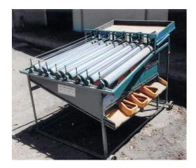
**5)** Technology description: The roller type fruit grader having four pairs of rollers (PVC pipes) of 100 mm diameter and 1500 mm length rotating (opposite and outward) at 80 rpm with adjustable diverging gap between each pairs of roller has been developed. The grader is useful for grading Nagpur mandarin, Sweet lime and sapota (spherical varieties) into 3 to 4 grades with 70 to 85 % grading efficiency.
