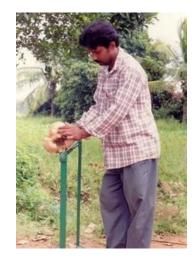
**5) Technology description:** The dehusking assembly consists of two sharp edged blades, one being stationary and the other movable - operated by a foot pedal through linkage mechanism. The twin-blades are mounted on a tubular stand. The unhusked coconut is pierced on the wedge like blade and then the foot pedal is pressed to split open and separate a portion of the husk. The operation is repeated 3-4 times until complete dehusking is done.
