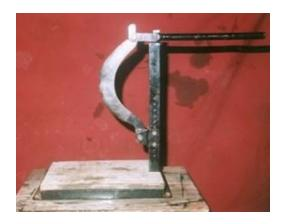
**5) Technology description:** Application/Use: For drinking tender nut water. Unit cost: Rs.3500/-. Output Capacity: 150 – 200 nuts/hr.
